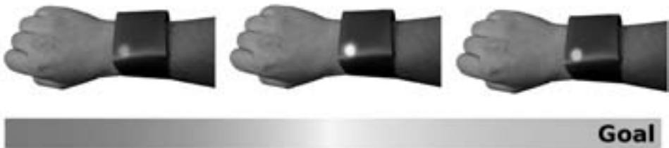
Fig. 5: Spectrum of colours displayed by device. From red (no daily activity) to green (daily goal achieved).
